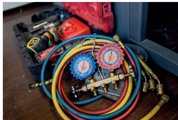
Picture 8: Manifold used for evacuating natural refrigerants, © Gianfranco Vivi, GIZ
