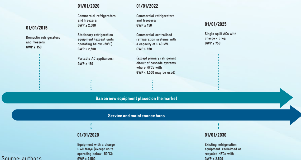
Figure 10: Overview of GWP limits according to EU F-gas Regulation
