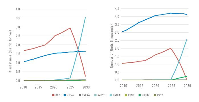
FIGURE 21: ESTIMATED END-OF-LIFE (EOL) REFRIGERANT BANKS (LEFT SIDE) AND EOL UNITS (RIGHT SIDE) IN GRENADA'S RAC SECTOR, 2010-2030
